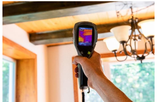
Thermal imaging showing the cold edges of a ceiling.
